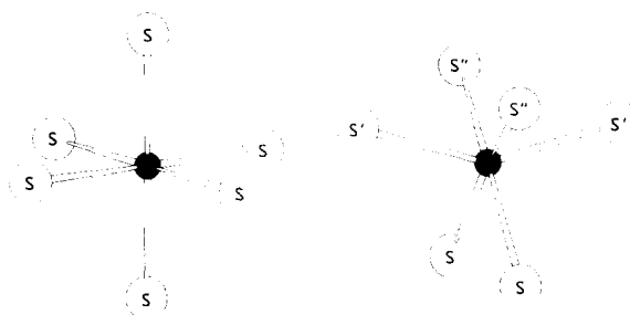
Fig. 3. Polyhedra of coordination in T-Yb 2 S 3 : [(Yb1)S 6 ] (left) and [(Yb2)S 6 ] (right).
